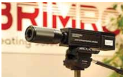
Figure 5. An integrated IR camera/acousto-optic tunable filter hyperspectral imaging system can activate optical taggants beyond the normal vision capabilities.
