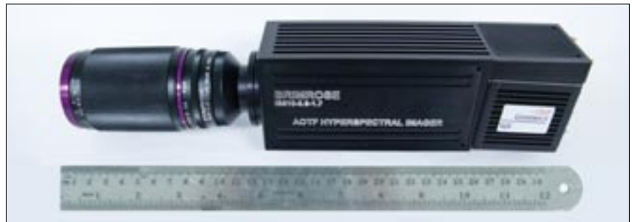
Figure 3. A Brimrose hyperspectral imager used for identifying optical taggants at unconventional wavelengths.
